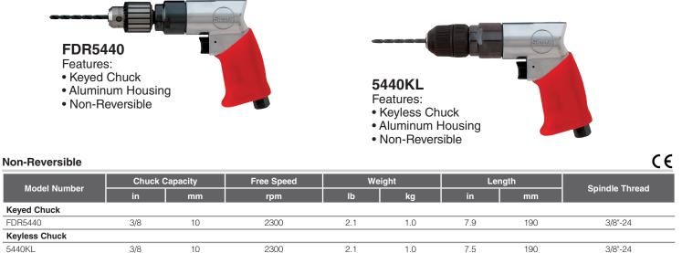
General: Air Inlet Size: 1/4" NPT • Recommended Hose Size: 3/8" (10 mm) • Performance rated @ 90 psig (6.2 bar) air pressure
