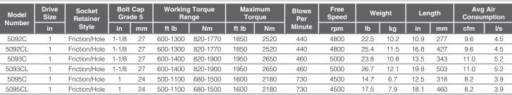
General: Air Inlet Size: 1/2" NPT • Recommended Hose Size: 1/2" (25 mm) • Performance rated @ 90 psig (6.2 bar) air pressure Standard Equipment: Parts List • Safety and Instruction Manual • D-Style Support Handle
